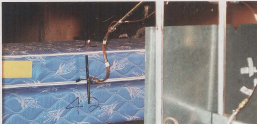
Burner positioning for TB603 test.
